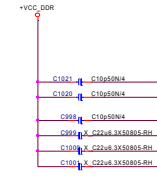
DDR4 I/O power decoupling caps.
